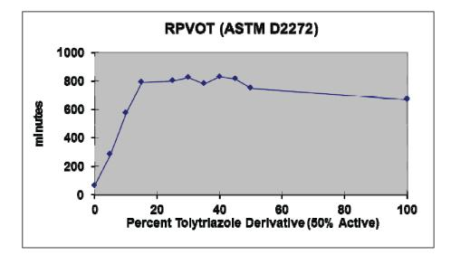
Figure 4 | RPVOT data for Group I base oils treated with variable proportions of an ashless dithiocarbamate and tolyltriazole derivative with all formulations containing a total of 0.7 mass percent of these two additives. All formulations contain 0.1 mass percent of succinic half-ester rust inhibitor. (*Courtesy of R.T. Vanderbilt Co., Inc.*)
