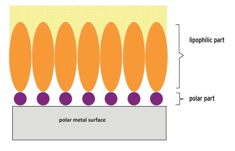
Figure 1 | Metal deactivators establish inactive barrier films through their polar part, which absorbs on the metal surface. On the opposite side, the lipophilic component interacts with the lubricant. (Courtesy of Rhein Chemie Rheinau GmbH)
