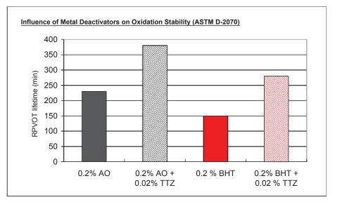
Figure 5 | A small treat rate (0.02%) of tolyltriazole (TTZ) improves the performance of an antioxidant (AO) and the phenolic antioxidant, butylated hydroxytoluene (BHT) in the RPVOT Test. (*Courtesy of Rhein Chemie Rheinau GmbH*)
